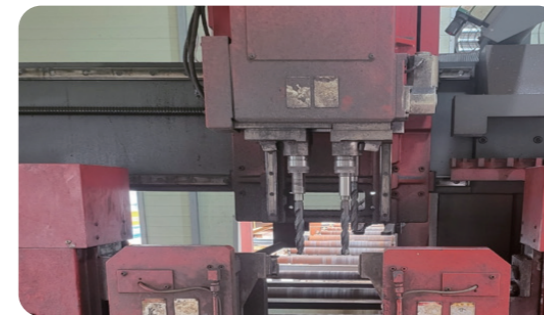
CNC 드릴머신 CNC Drill MC / 1대 PC1500N / MAX.80mm
