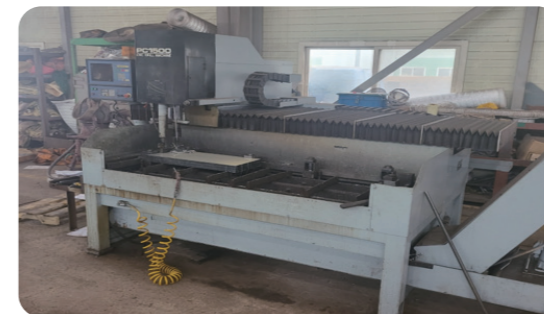
CNC 드릴머신 CNC Drill MC / 1대 PC1500N / MAX.80mm
