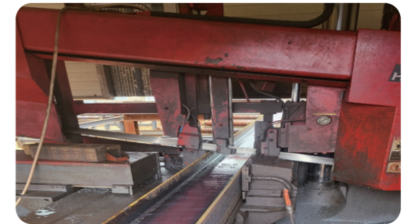
밴드쇼우 Band Saw / 3대 H600(2대), H-700CNC(1대) / 65*25 - 700*400
